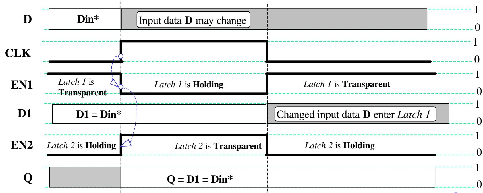
The state of the flip-flop's output  $Q$  copies input  $D$  when the positive edge of the clock  $CLK$  occurs
