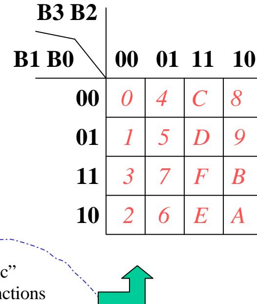
As we are using ad-hoc “binary-hex logic” equations, (i.e. binary S... outputs as functions of hex variables) it will be useful in this case to have hex-labeled Karnaugh map, instead of the usual 2-D (i.e. two dimensional) binary labeled K maps. This will allow for a more convenient mapping of the “binary-hex” logic equations onto the K-maps.
