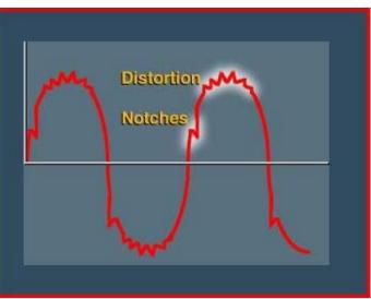
C Operations using ASD's in the vacinity of sensitive electronic equipment should consider including either an isolation transformer, or line reactors on the input of the drive to protect the other equipment from this potential problem.
