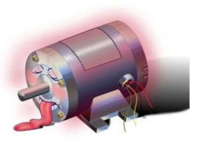
As a rule of thumb, you can generally take a fully loaded Class B insulation motor down to 50 percent speed on constant torque loads without overheating.
