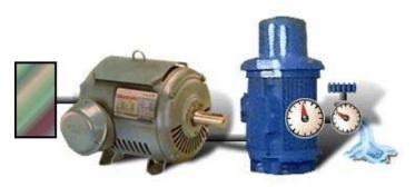
Do not assume 75 percent flow equals 75 percent load. For fans and pumps, the load varies as the cube of the fan or pump speed.
