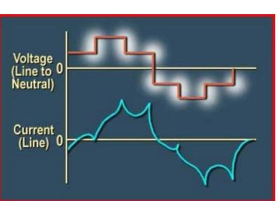
During low speed operation (below 15-20 Hz) cogging can be a problem where the jerky motion of the motor shaft can create problems for bearings, gears, or gear reducers.
