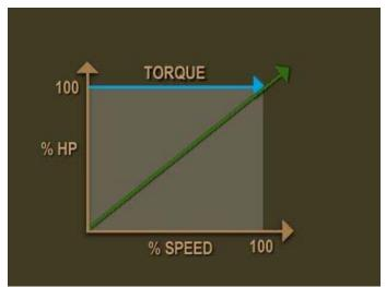
Constant torque loads include most conveyors, positive displacement and reciprocating pumps, and compressors.
